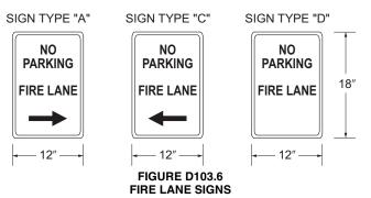
**D103.6.1 Roads 20 to 26 feet in width.** Fire lane signs as specified in Section D103.6 shall be posted on both sides of fire apparatus access roads that are 20 to 26 feet wide (6096 to 7925 mm).
